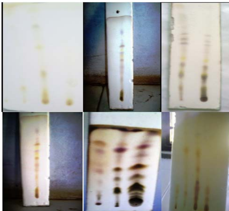
Fig 3.1: Thin layer chromatography qualitative analyses of six fractions against Indigofera tinctoria plant flower extract
