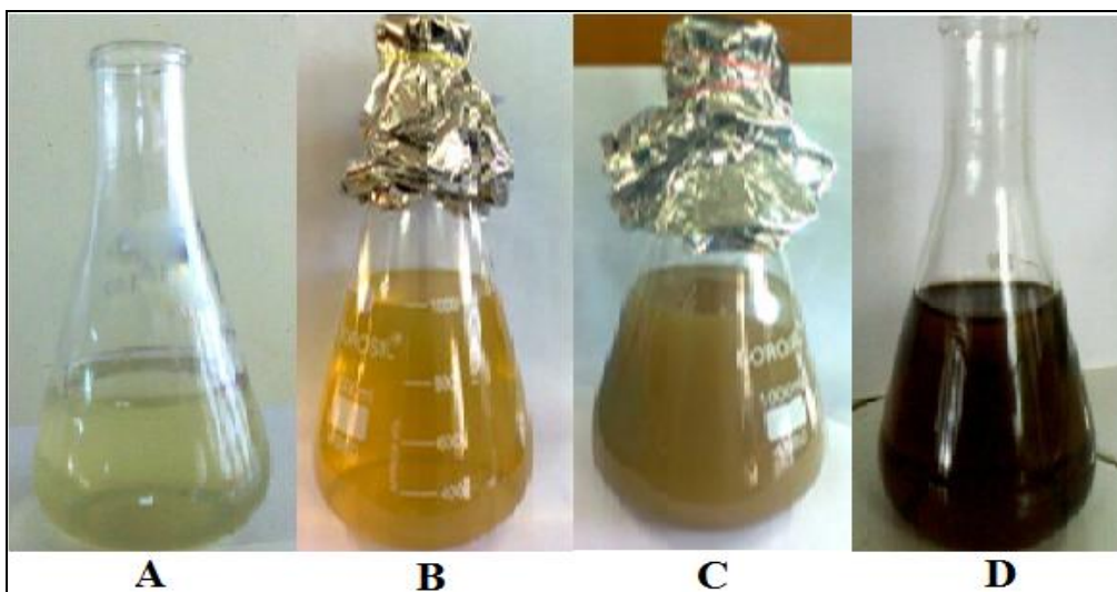
A-D: A. indica Leaf extract showing the colour change in the synthesis silver nanoparticles on incubation time.
