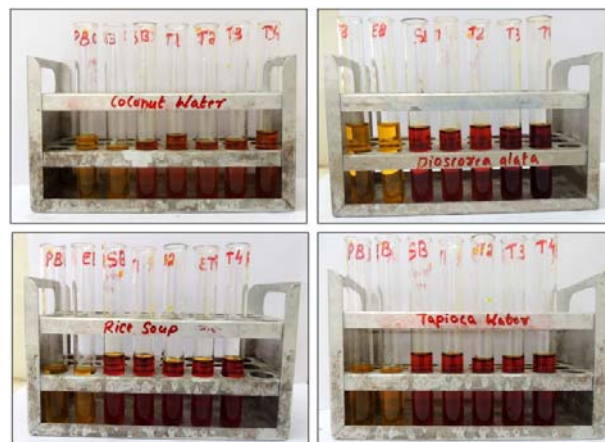
Fig 2: Amylase produced by submerged fermentation using various substrates and their enzymatic activity, coconut water (top left); white yam water (top right); rice water (middle left); tapioca water (middle right).
