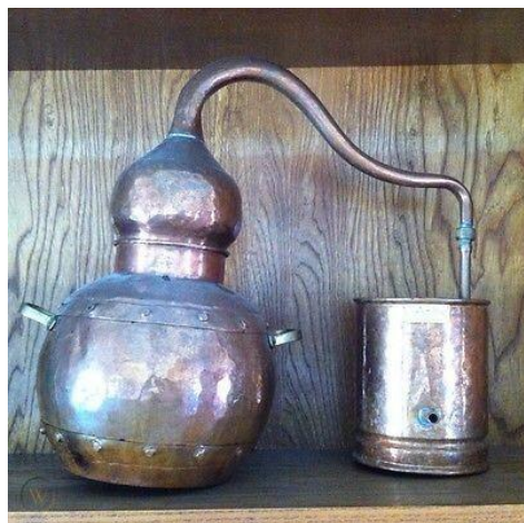
Picture 2: Alembic has been used to extract essential oil from Damask Rose
