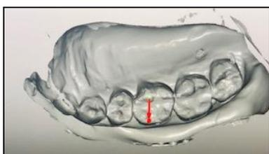
**Fig 5:** Measurement of the distance between two fixed points on a scanned sectional addition silicone impression
